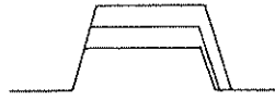
Fig. 6-3. Pulse duration remains constant when the amplitude is varied at equal values of rise and fall time
